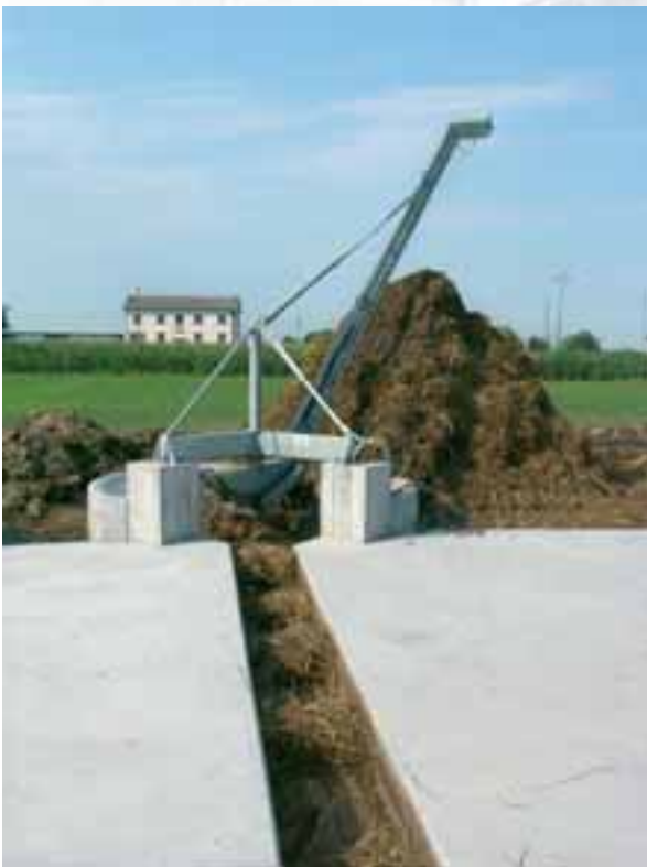
EGN model Elevator with 180° swivel for manure piling. Belt lengths 6 – 8 – 10 metres
