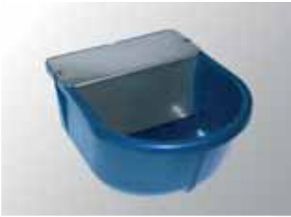
F14 - Constant level drinker with built-in float. Capacity 6 litres. Drain plug for cleaning.
